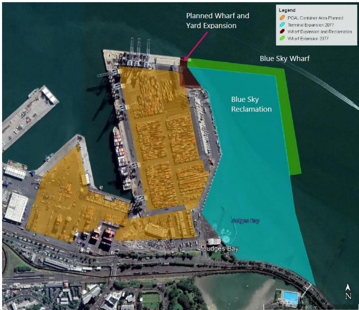
Figure 6 POAL – A concept for required container terminal area, assuming unconstrained expansion to 2079
