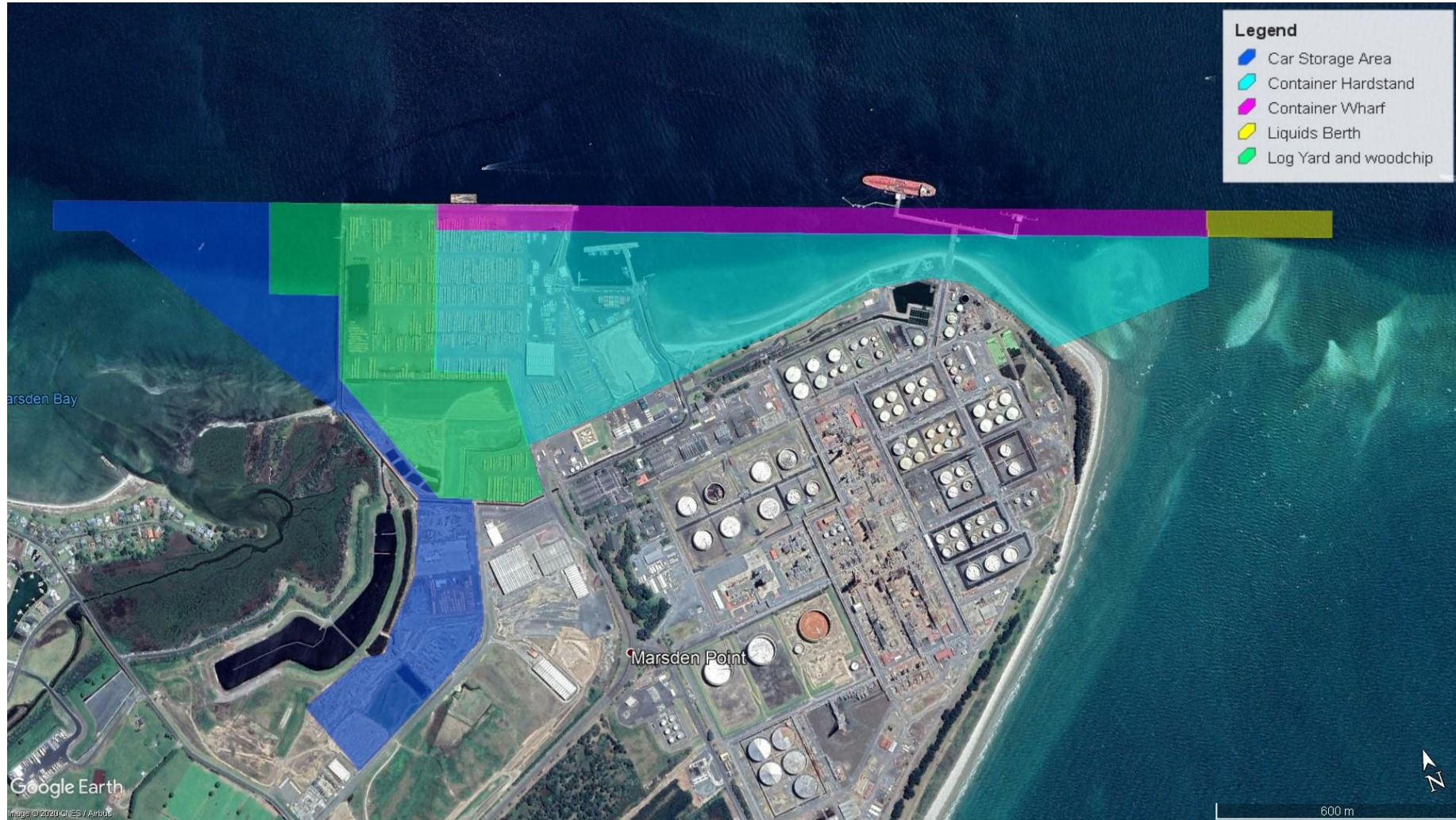
Figure 7 Northport expansion – concept layout for forecast freight task, 2079
