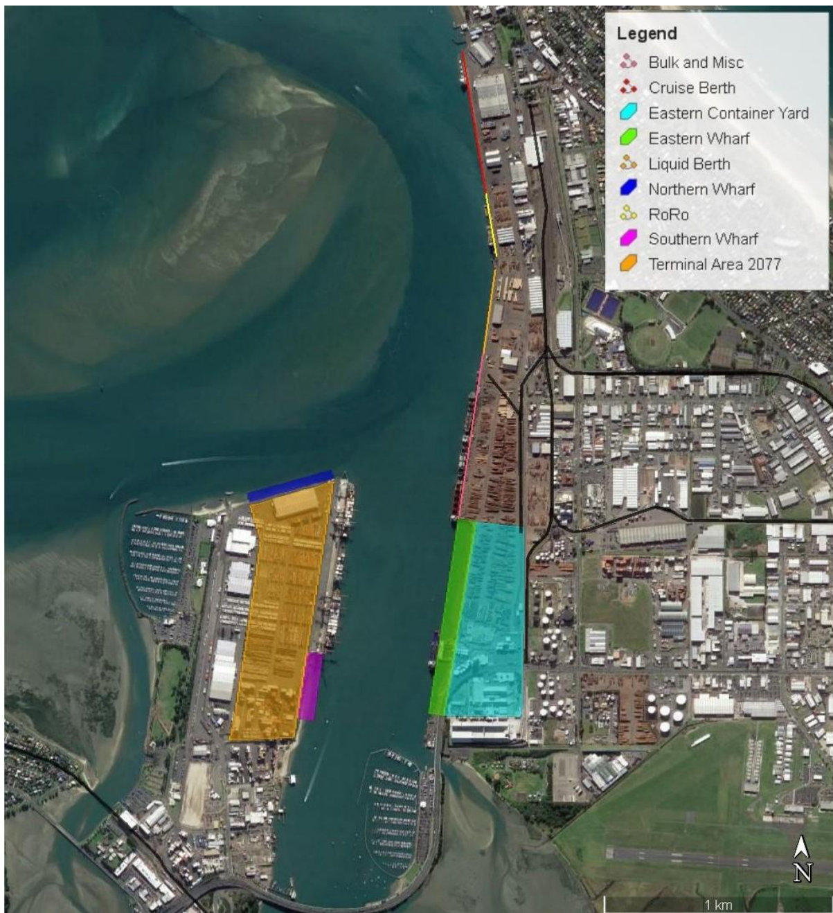
Figure 10 Port of Tauranga expansion under split option – concept layout for forecast freight task, 2079
