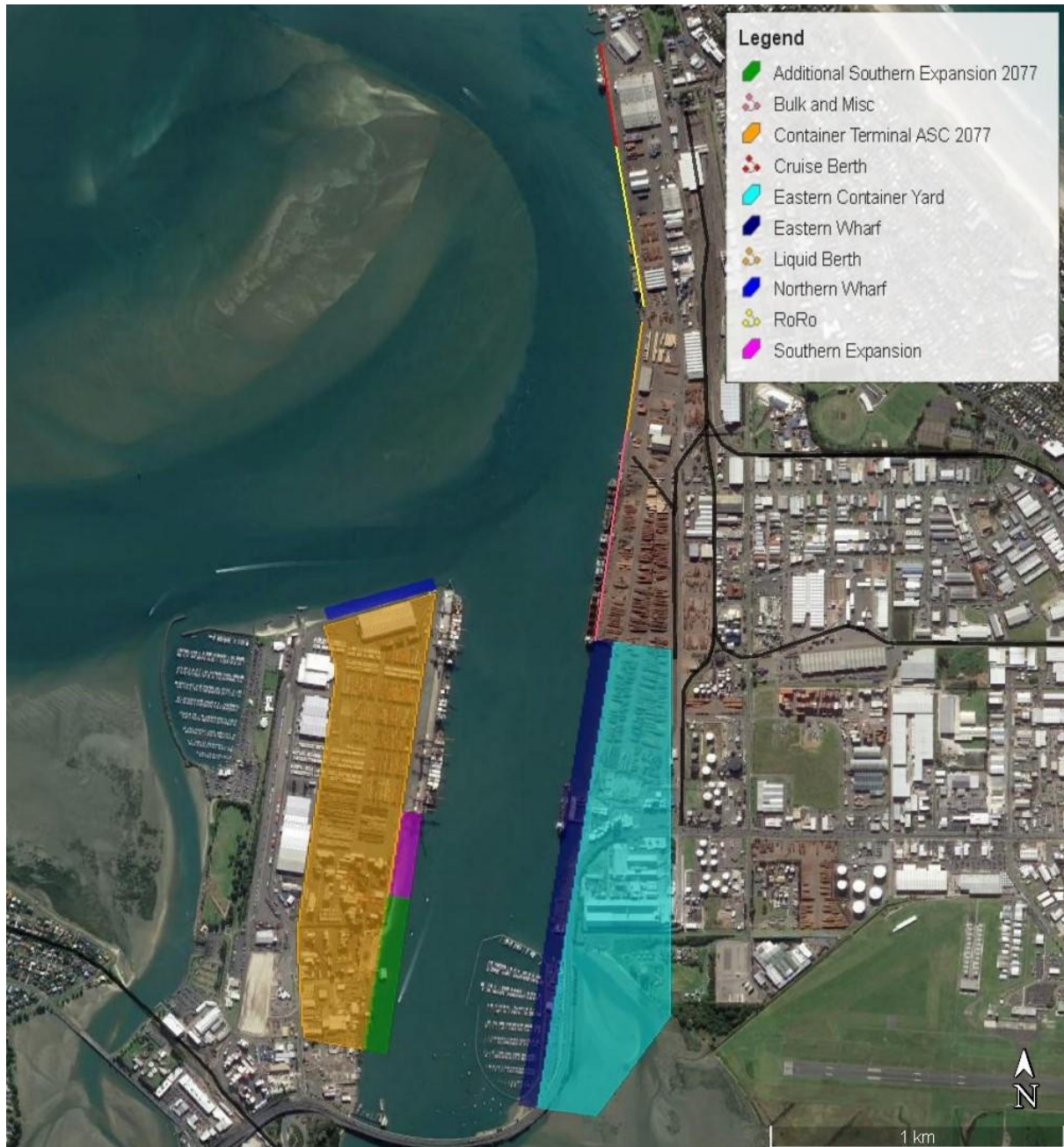
Figure 8 Port of Tauranga expansion – concept layout for forecast freight task, 2079
