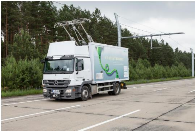
Figure 8: Hybrid electric truck under a catenary in a Siemens pilot project
