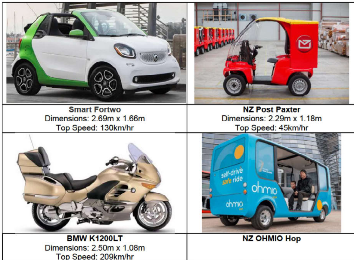
Figure 2 – microCAR models vs BMW K1200L
